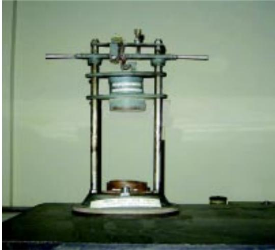
**FIG. 6 : AGGREGATE IMPACT TEST MACHINE**
